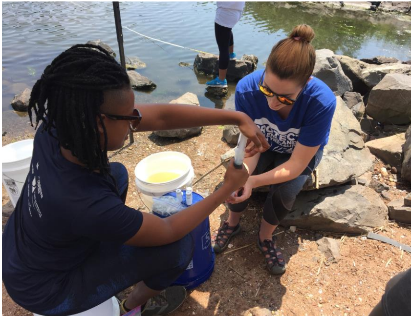
Figure 25. Billion Oyster Project Research Assistant Technician J Robinson and Scientist Liz Burmester using syringe filters to collect dissolved inorganic nutrient samples at Lemon Creek Lagoon in August 2017. (Photo: Cheryl Bennett, The Nature Conservancy)
