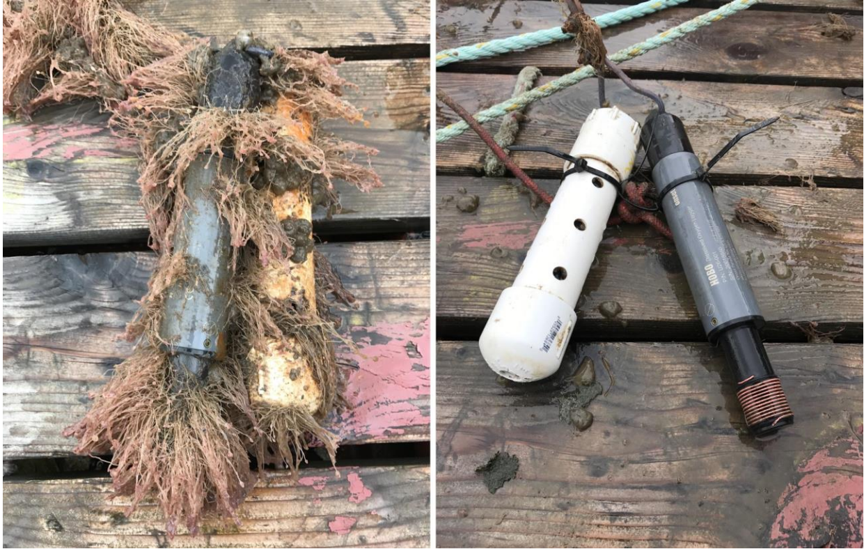
Figure 15. Water quality loggers on Governors Island EcoDock before ( left ) and after ( right ) removal of fouling organisms, offloading of data and recalibration. (Photos: Mike McCann, The Nature Conservancy)
