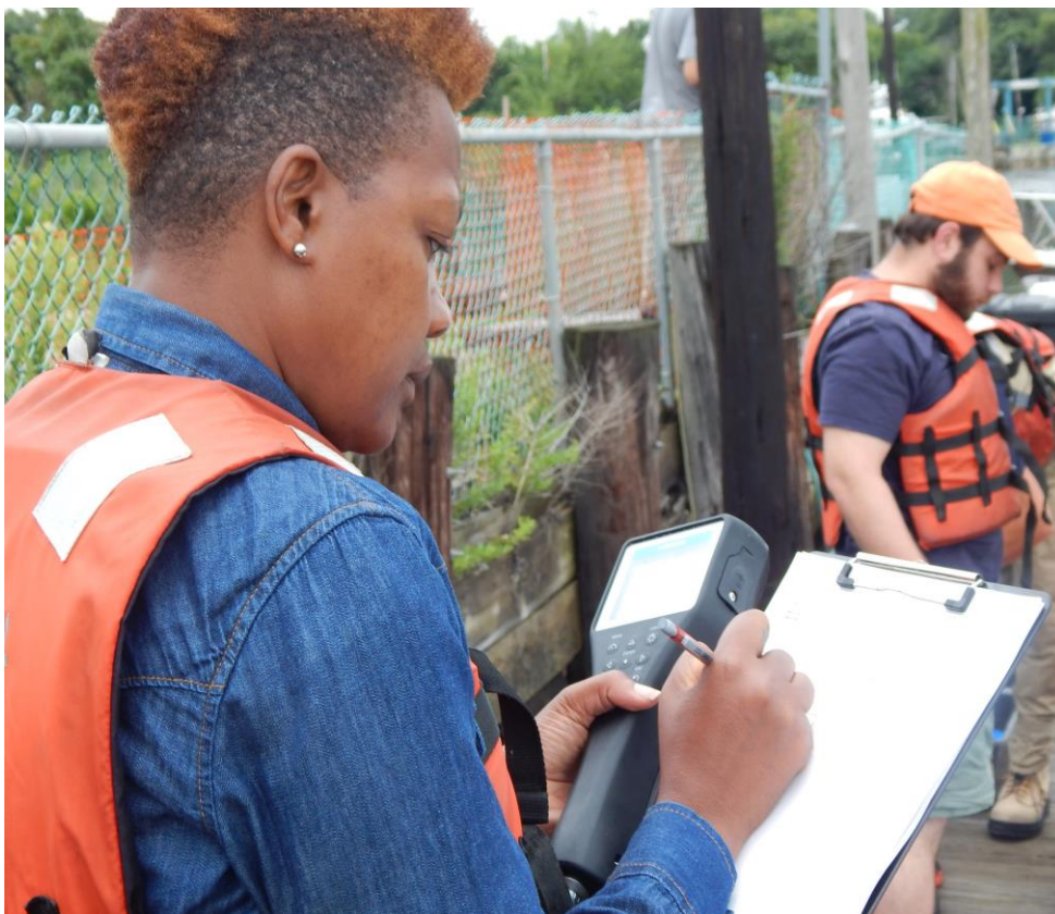
Figure 12. TNC Summer Fellow Cheryl Bennett using the Horiba U-52 to record water quality at the Lemon Creek Nursery in August 2017. (Photo: Robina Taliaferrow, Billion Oyster Project)
